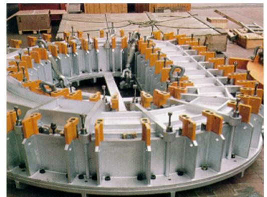
***Coil inside impregnation mould***
