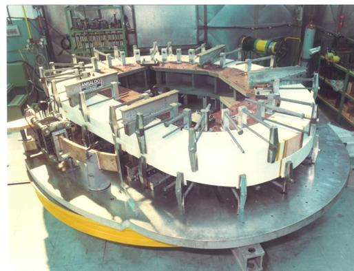
***Turns assembly on winding table***
